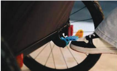
The parking brake can be released by lifting the foot on the foot brake.
