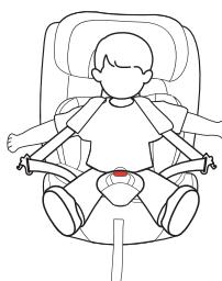
1. Loosen the seat belt to the fullest extent, then unlock the buckle and place it on either side of the seat, as shown in the picture.
