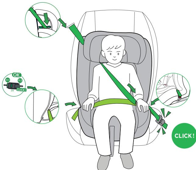
1. To secure the child in this way, the 5-point harness must be hidden first (see 4-7 for details).
