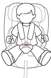
2. Insert the left and right latches into the buckle and hear a "click" sound, indicating that the buckle is fastened. Press the adjustable belt button to adjust and tighten the shoulder strap, while ensuring that the child's shoulders are comfortable (a finger space should be there between the seat belt and the child).
