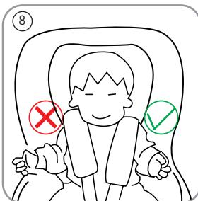
2. Correctly adjusting the headrest can ensure the best protection for your child in the car seat. The headrest must be adjusted to the position that the shoulder strap is compatible with the height of a child's shoulders or slightly higher. The straps must be located at shoulder height or slightly above the child's shoulder height. The shoulder strap should not be behind the child or over the ears.
